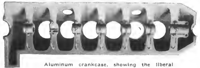
Aluminum crankcase, showing the liberal dimensions of the seven main bearings and the direct high pressure oil leads
